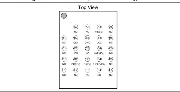
Figure 1d. W25Q01JV Ball Assignments, 24-ball TFBGA 8x6-mm (Package Code TB)
