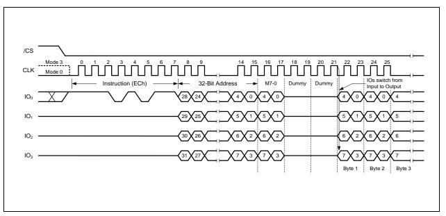
Figure 28. Fast Read Quad I/O w/ 4-Byte Addr. (M7-M0 should be set to Fxh)
