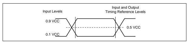
Figure 66. AC Measurement I/O Waveform
