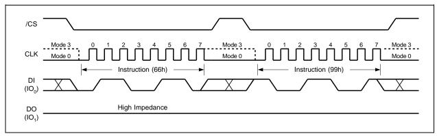
Figure 60. Enable Reset and Reset Instruction Sequence
