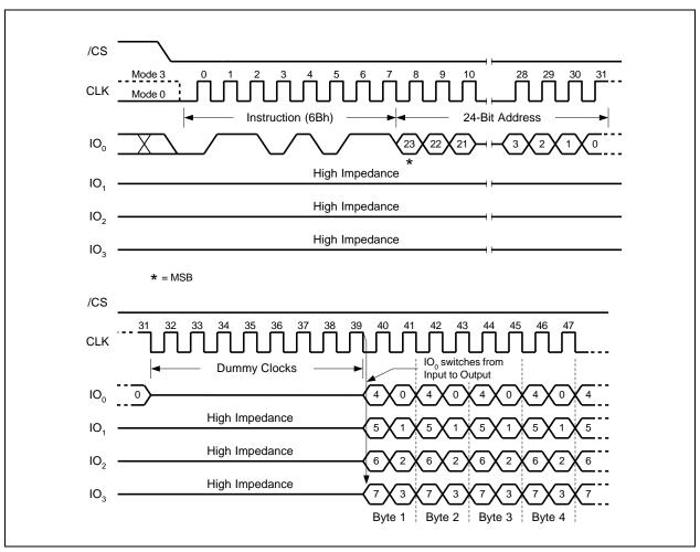
Figure 21. Fast Read Quad Output Instruction
