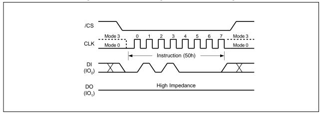
Figure 6. Write Enable for Volatile Status Register Instruction
