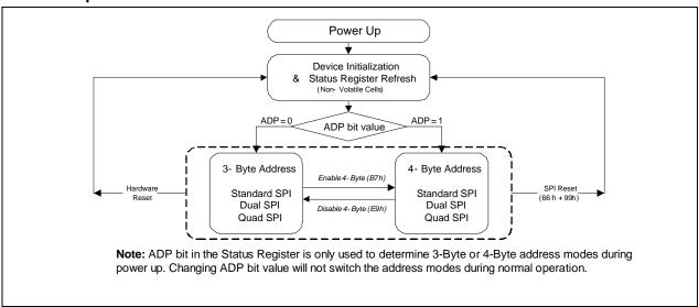
Figure 3. W25Q01JV Serial Flash Memory Operation Diagram
