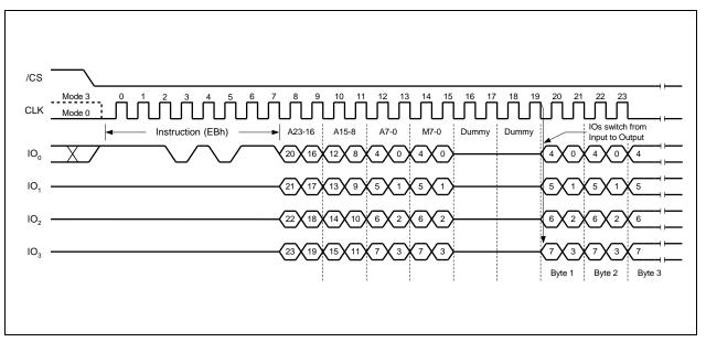
Figure 26a. Fast Read Quad I/O (M7-M0 should be set to Fxh)
