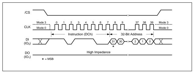
Figure 40. 64KB Block Erase with 4-Byte Address Instruction
