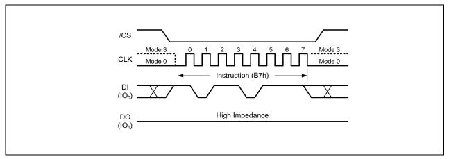
Figure 12. Enter 4-Byte Address Mode instruction
