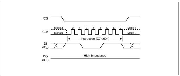
Figure 41. Chip Erase Instruction Sequence Diagram
