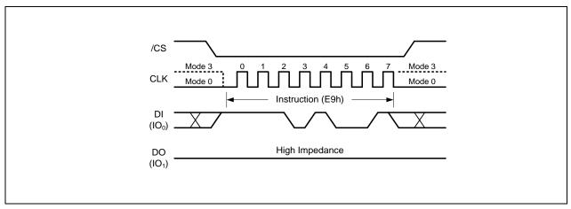
Figure 13. Exit 4-Byte Address Mode instruction
