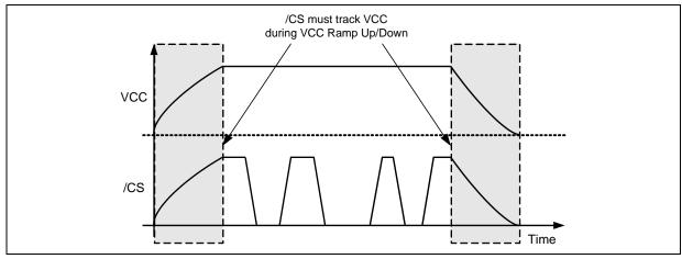
Figure 65b. Power-up, Power-Down Requirement
