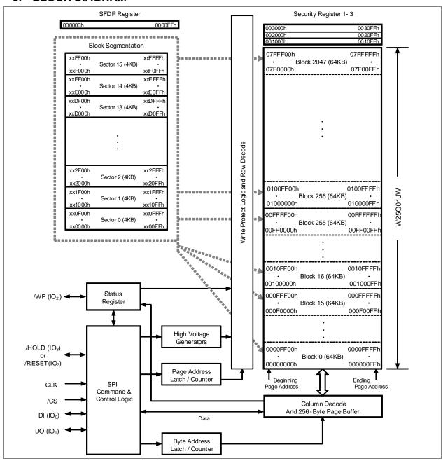
Figure 2. W25Q01JV Serial Flash Memory Block Diagram
