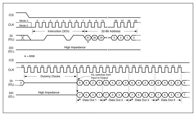
Figure 20. Fast Read Dual Output with 4-Byte Address Instruction
