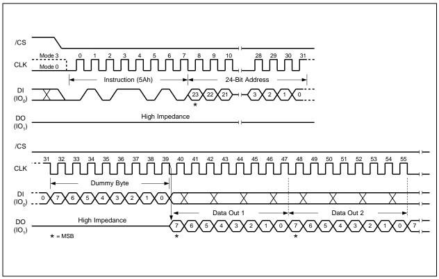
Figure 51. Read SFDP Register Instruction Sequence Diagram
