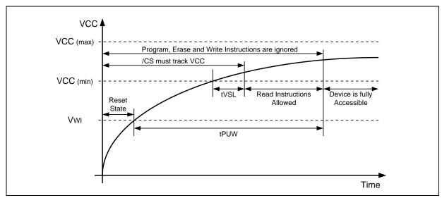
Figure 65a. Power-up Timing and Voltage Levels
